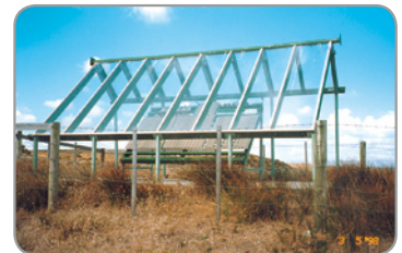
The sheltered rack simulates under-roof and non-rain washed situations
