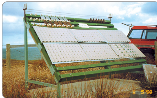
Each outdoor site contains two exposure racks. The open rack simulates conditions on a roof.
