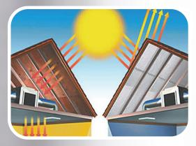
There are three types of heat transfers: conduction, convection and radiation. Nearly 87% of the total building heat is transferred via this radiation. In this way, radiation is the most powerful cause of heat gain in any building.
